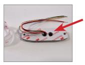
Ensure vent hole is aligned properly
